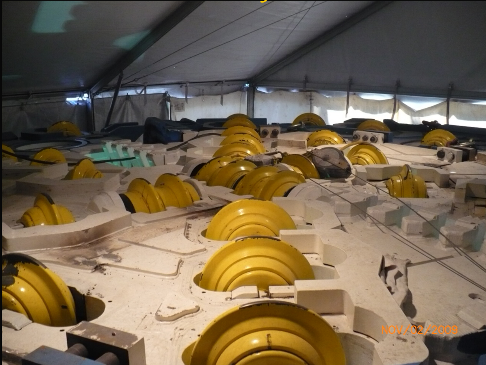
Cutter Head - Welding in temperature controlled tent
